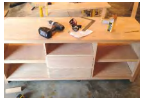
STEP 15. Next, cut and edge the left and right shelves with finishing trim, then, measure and cut the drawer fronts to the size of the openings. I opted for two drawers at the bottom and left the top open for a digital box and/or DVD player
